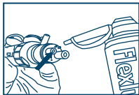
Fig. 9 - Lubrificação Conexão Midwest. Fig. 9 - Midwest Connection Lubrication. Fig. 9 - Lubricación Conexión Midwest.
